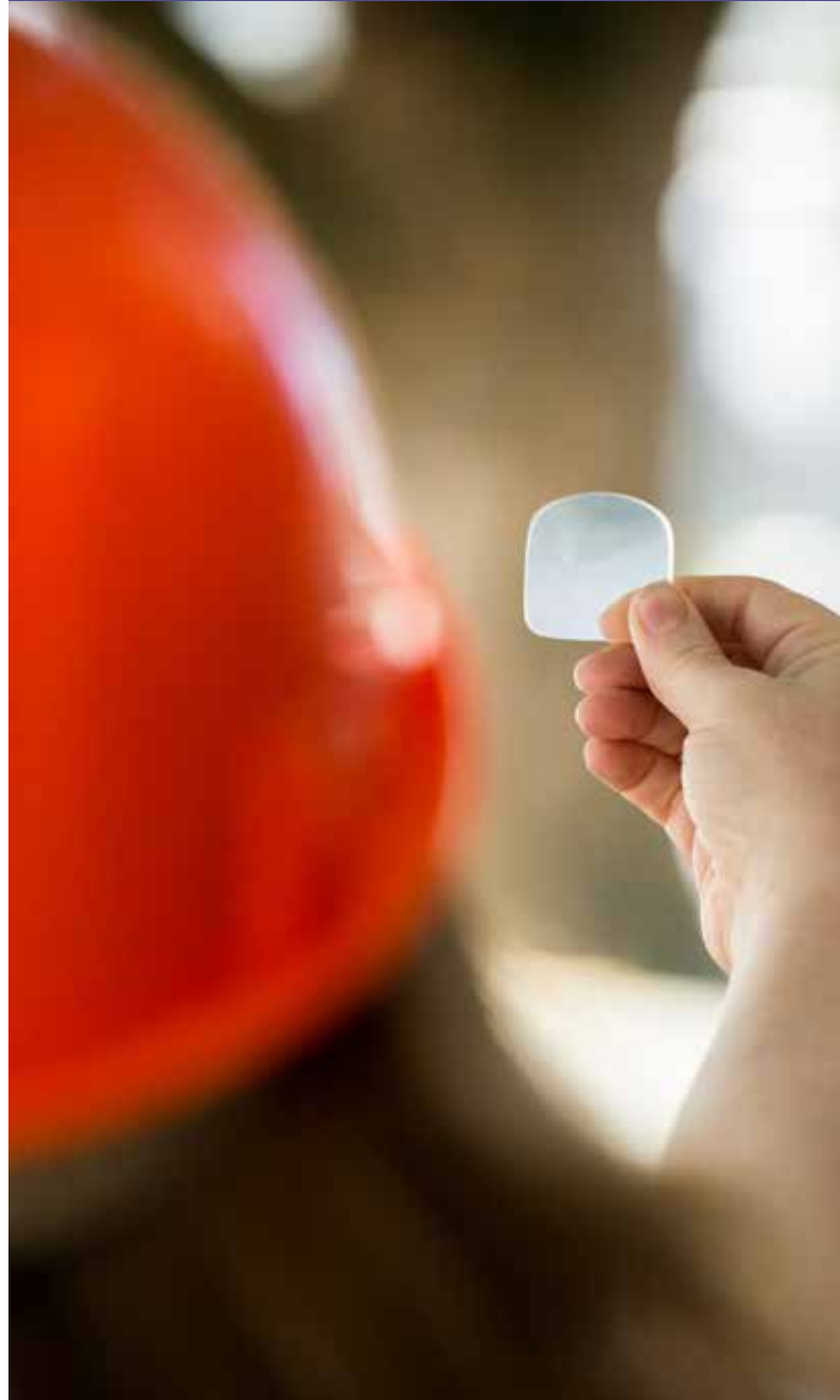
ABOVE Beth looks at a prism used to measure basal area at a timber cruise plot. Basal area is used in the calculation of an estimate of volume.
